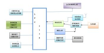
Figure 2. Block Diagram
