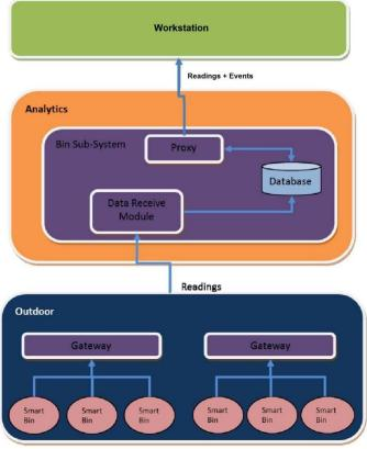
Figure 2. Smart-Bin system architecture
