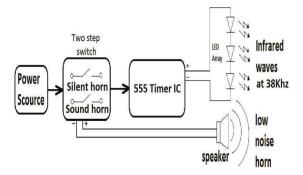
Figure 2. Transmitter block diagram
