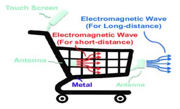
Figure 2. RFID module installed on the SSC
