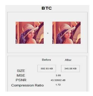
Figure 1. Compressed result using BTC
