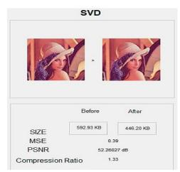
**Figure 3.** Compressed result using SVD We can see that the image is compressed from the size 592.93 KB is reduced by the SVD to 446.20 KB.
