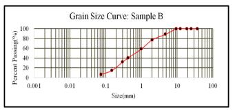
**Figure 3:** Mean particle size distribution curve for Samples from the Farmington Formation
