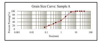
Figure 2: Mean particle size distribution curve for Samples from the Paynesville Sandstone
