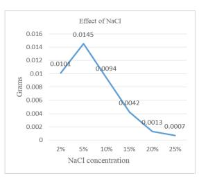
Fig. 7 : Effect of NaCl on production of PHB
