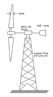
Figure 4 : Horizontal – Axial Machines
