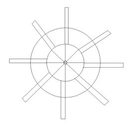
Figure 5: Horizontal axis multibladed type
