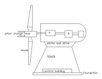
Figure 3: The transmission system of WEC
