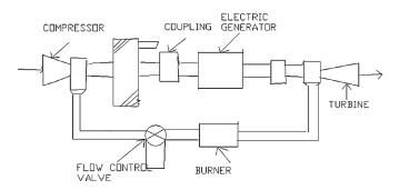
Figure 10 : The mode of operation
