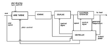
Figure 2. The main components of a WECS
