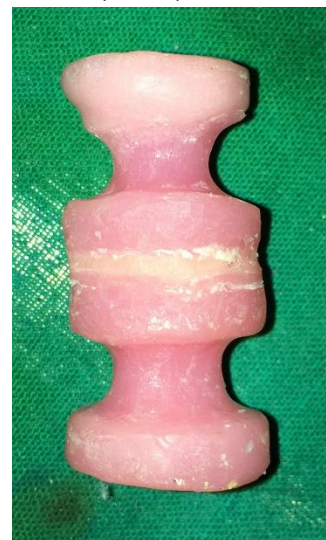
Figure 2: Dumbbell shaped heat cure acrylic resin specimens with soft liner
