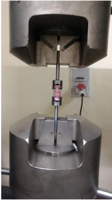
Figure 3: Testing of the specimens for tensile bond strength
