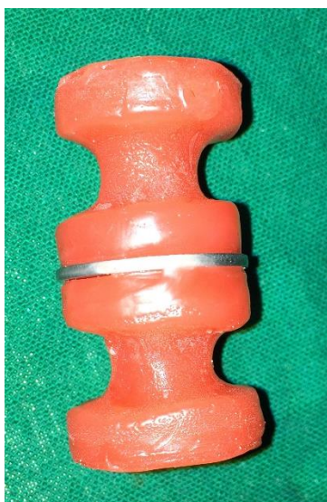
Figure 1: Dumbbell shaped wax pattern
