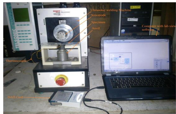
Fig 25. Experimental set up with temperature measurement attachment
