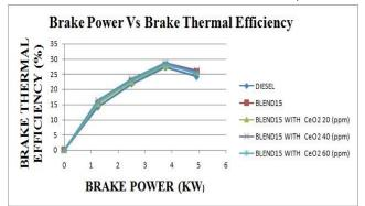
Fig 8. Brake Power Vs Brake Thermal Efficiency
