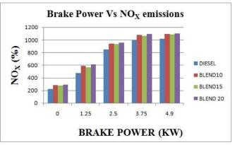
Fig 7. Brake Power Vs NOx emissions
