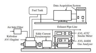
Fig.1. Schematic diagram of experimental set up
