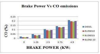
Fig 6. Brake Power Vs CO emissions
