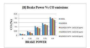
**Fig 11:** Brake Power Vs CO emissions Fig 11 shows the graph between brake power and co emissions At load 9kg, Carbon Monoxide emissions for Diesel, Blend 15, Blend15+CeO<sub>2</sub>20ppm, B15+CeO<sub>2</sub>40ppm and B15+CeO<sub>2</sub>60ppm are 0.141%, 0.123%, 0.132%, 0.121% and 0.117% respectively.
