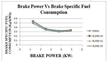
Fig 4: Brake Power Vs Brake Specific Fuel Consumption
