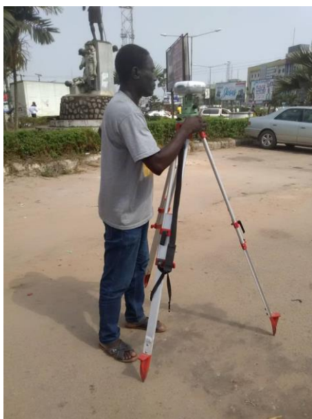
Figure 5: Rover Receiver at One of the Chosen Points at the Frontage of Central Baptist Church, Ring Road
