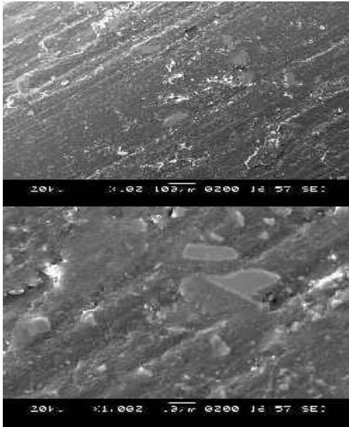
Figure 3: SEM Micrographs of 5wt% Al 2 O 3 and 5wt% SiC Epoxy Composite
