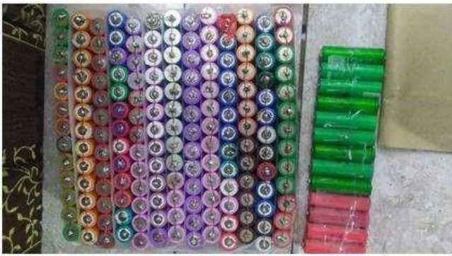
Fig 4. LITHIUM-ION BATTERY PACK
