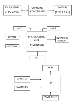
It is also interfaced to an ultrasonic sensor for object detection. The ATMEGA328 controller moves the vehicle motors in the forward direction in case no obstacle detected. On obstacle detection, the ultrasonic sensor monitors it and the controller and thus stops the grass cutter motor so as to avoid any damage to the object/human/animal. The controller then turns the robotic vehicle off until it gets clear of the object and then moves the grass cutter in a forward direction again.
