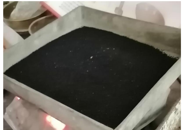
Fig.1- Sample of Rubber crumb of specific grain size
