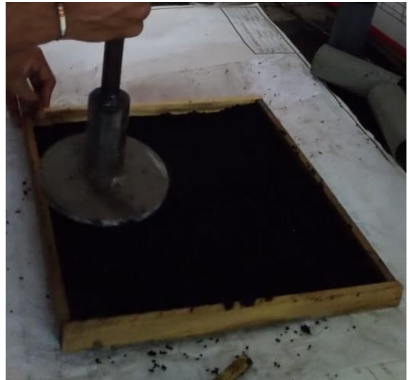
Fig.4- preparing sheet by providing compaction
