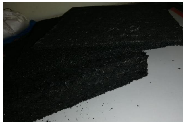
Fig.5- Sample of sheet after de-moulding
