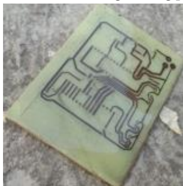
Figure 6.7.3 PCB after etching process
