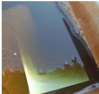
Figure 6.7.2 PCB during etching process
