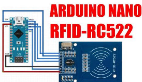
Figure 6.3 Arduino Nano to RFID
