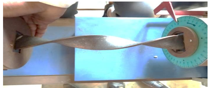
Fig (7) Specimen in torsion testing machine
