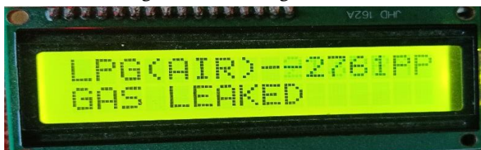
Fig. 5.2 Leakage Gas in Air (PPM)
