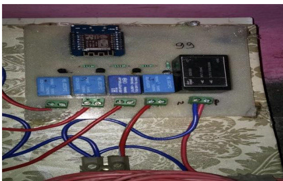
Fig: Circuit connections with 4 relays.
