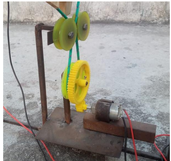
Figure 5 : Solar panel tracking using dc motor.
