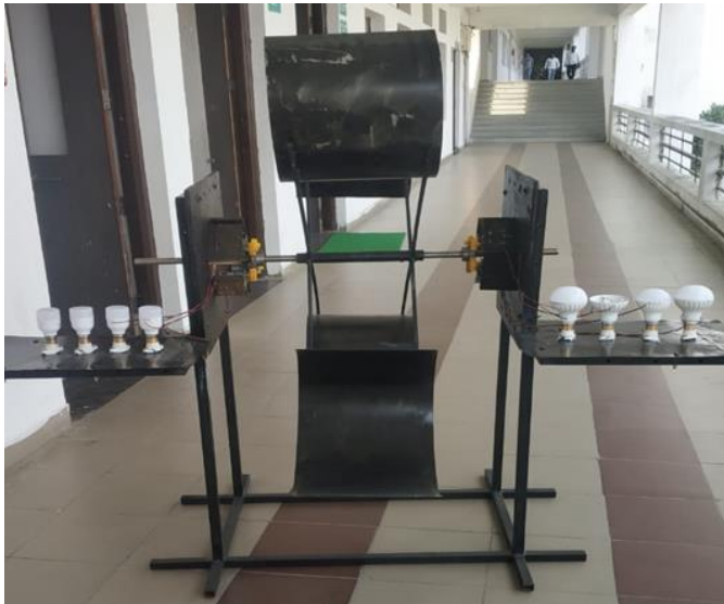
Fig.8 :- Modern Savonius With Arm Gear Based Structure model
