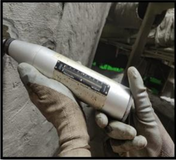
Fig 2: - Rebound Hammer Test
