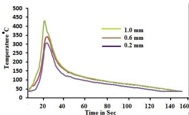
Fig.4.7 Effect of Amplitude on Temperature profile
