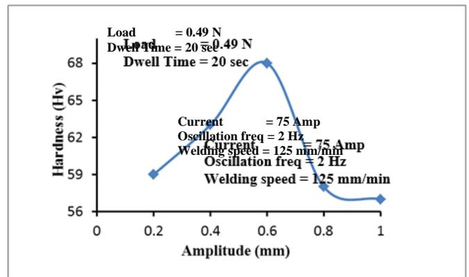
**Fig 3.5 Effect of arc amplitude on fusion zone hardness graph**
