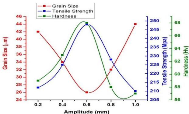
**Fig 4.6** Effect of arc amplitude on grain size, microhardness and tensile strength
