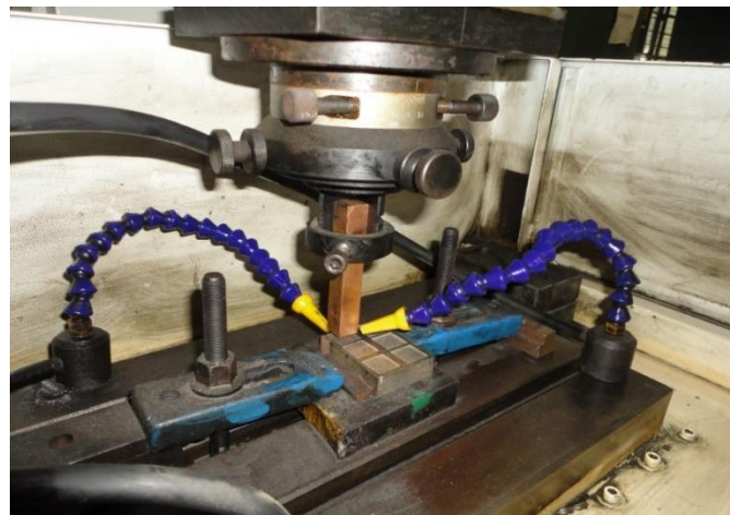
Fig 6: Positioning of workpiece and tool using fixtures
