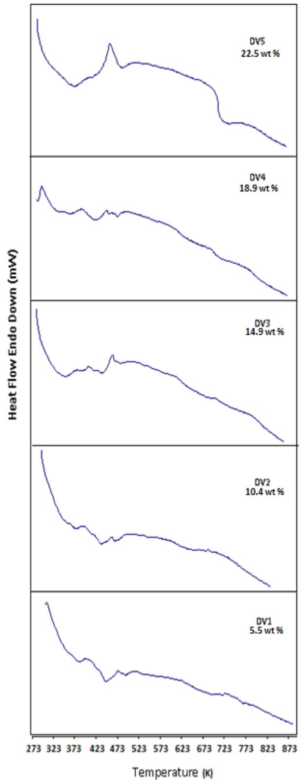
Fig.4: DTA Curve for Iodine doped PTh-PVAc films
