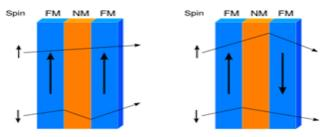
The reason for the changing electrical resistance is that the spin dependence of an electron transport, that affects the scattering rates at film interfaces for spinup (spin parallel to layer magnetization) and spindown (spin antiparallel to layer magnetization) electrons[12].
