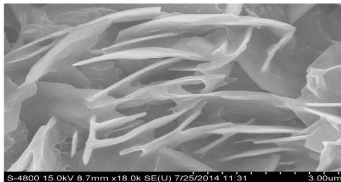
Fig. 3 FE-SEM micrograph of LiAl<sub>0.97</sub>B<sub>2</sub>O<sub>5</sub>:0.03Eu<sup>2+</sup> phosphor.
