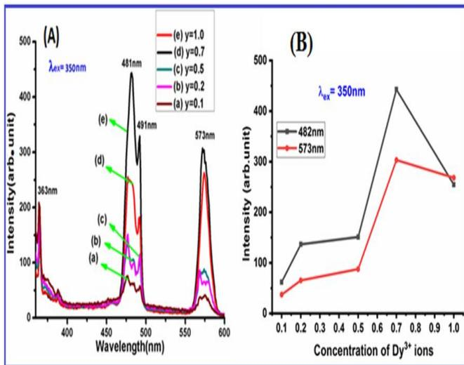
**Figure 2 (A)** PL emission spectrum of La<sub>2</sub>(MoO<sub>4</sub>)<sub>3</sub>:xDy<sup>3+</sup> (x = 0.1, 0.2, 0.5, 0.7, 1.0mol%)phosphor under 350nm excitation wavelength and **Figure 2 (B)**Variation in PL emission intensity with concentration of Eu<sup>3+</sup> ions
