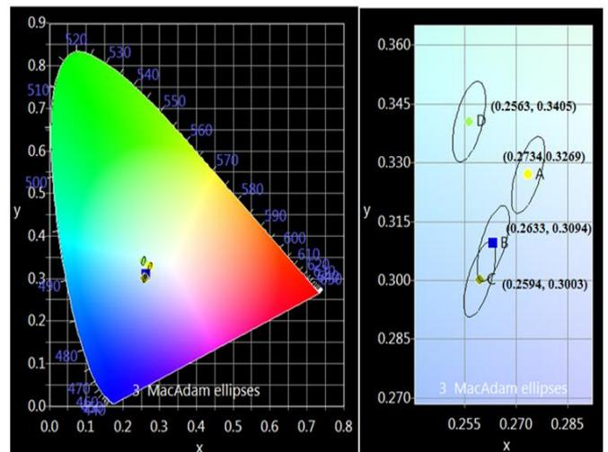
**Figure 5:**CIE chromaticity Diagram of La<sub>2</sub>(MoO<sub>4</sub>)<sub>3</sub>:0.7mol%Dy<sup>3+</sup> phosphors at different excitation wavelength
