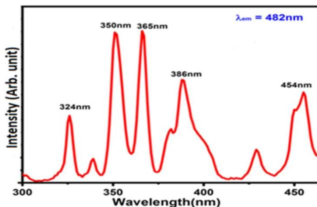
**Figure 1: PL excitation spectrum of Dy<sup>3+</sup> activated La<sub>2</sub>(MoO<sub>4</sub>)<sub>3</sub>phosphor under 482nm emission wavelength**
