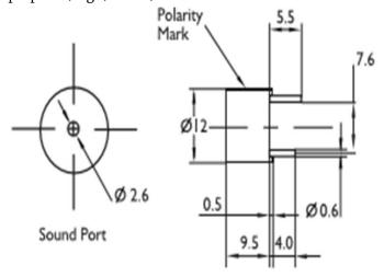
Dimensions : Millimetres Tolerance : ±0.5mm
