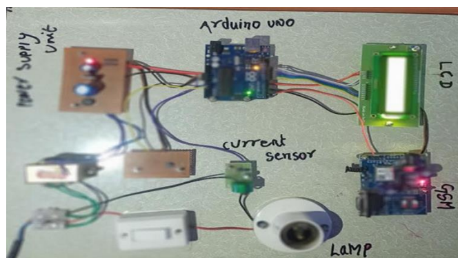
Figure 3 Prototype model of Smart Electricity Meter
