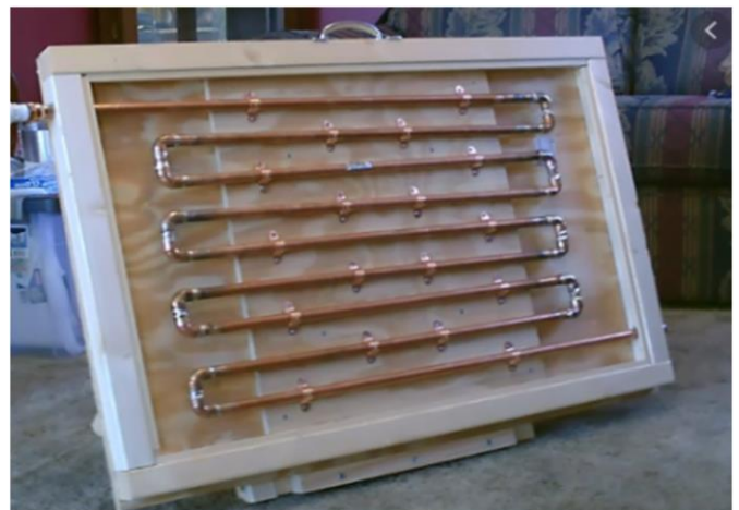
Figure 2: Cooling system using copper pipe
