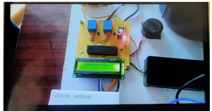
Fig 7: Display of the identified person in LCD
