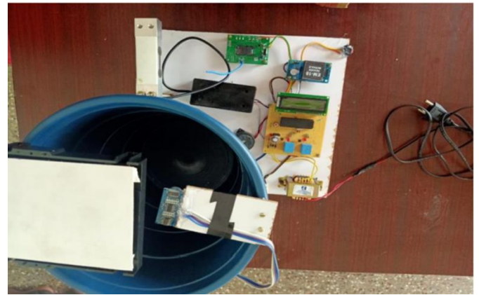
Fig 6: Trash bin with ultrasonic sensor.
