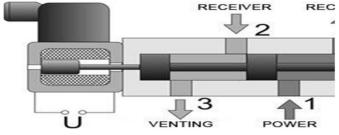
The directional valve is one of the important parts of a pneumatic system.
