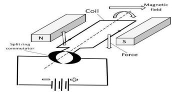
When a motor is in operation, it develops torque. This torque can produce mechanical rotation. DC motors are also like generators classified into shunt wound or series wound or compound wound motors.
