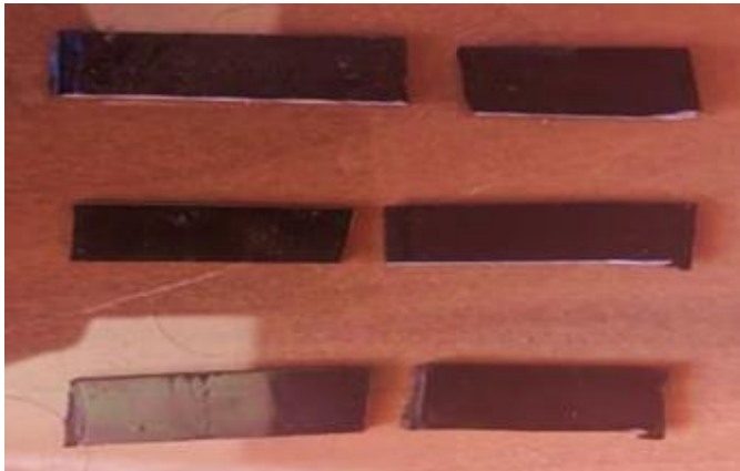
Fig 3.3 Typical specimen after impact test
