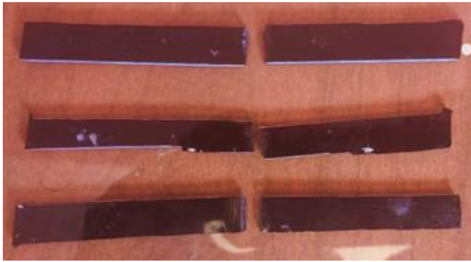
Fig 3.2 Typical specimen after flexural test
