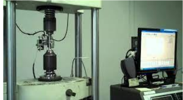
Fig 2.1 Tensile test on UTM
