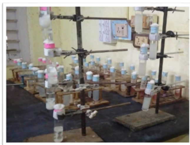
Fig. 1 Experimental set-up with working reaction during crystal growth in test tube.
