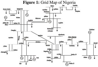
Figure 2: Single line diagram of the Nigerian Power grid
