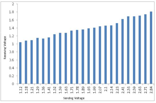
Figure 3: Variation of Receiving End Voltage with Sending Voltage
