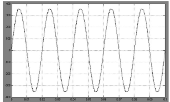
Fig. 5. O/P Double SPWM Voltage Waveform
