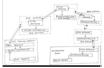
All these information from the base station is transferred to the intersectionpoint .The intersection point consists of the microcontroller and servo motor.The servo motor here act as the swith.The intersection point is nothing but the gate.The process here is when the information about the train is passed the servo motor act accordingly and the gate open or close based on the command.
