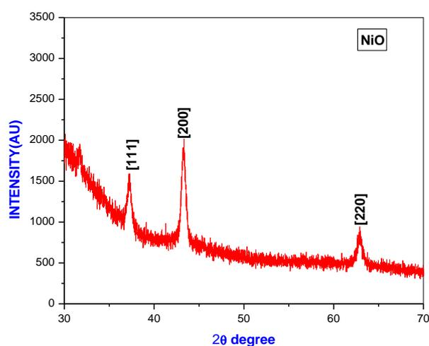
Figure 1 XRD pattern of NiO Thin Film electrode.
