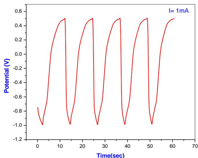
**Figure 6: the charge–discharge measurements of NiO electrode in 0.1M KOH electrolyte**
