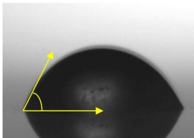
**Fig.4 Contact angle image of NiO film electrode**
