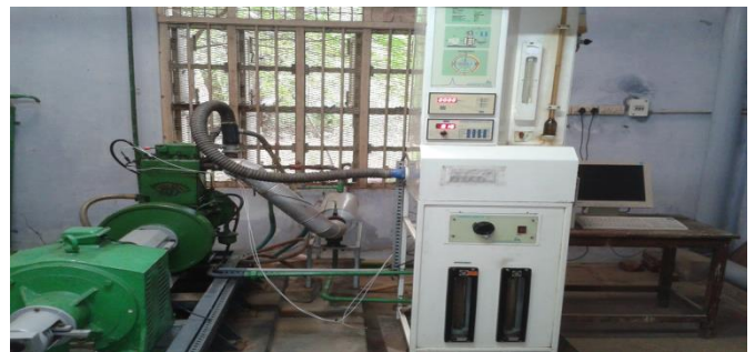
Fig 2: Single cylinder four stroke diesel engine test rig.
