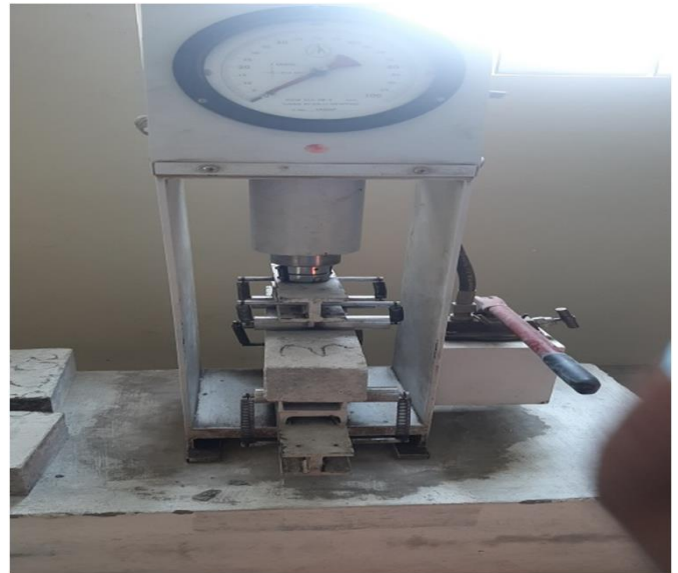
Fig. 6 Flexural Strength Test
