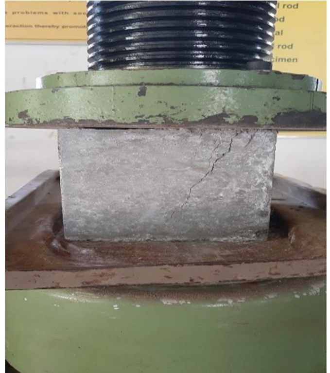
Fig. 3 Compressive Strength Test
