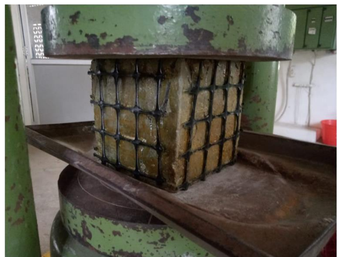
Fig. 8 RETROFITTING OF CUBE
