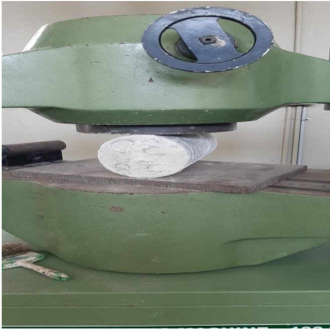
Fig. 6 Flexural Strength Test
