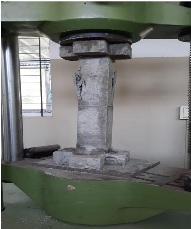
Fig. 4 Buckling of column
