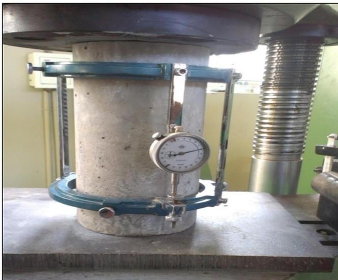
Fig. 9 Modulus of Elasticity Test
