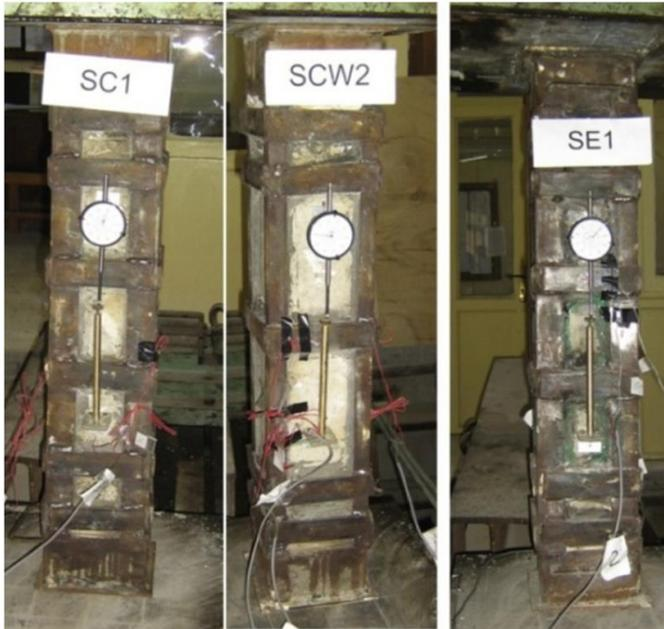
Both the ends of the specimens were protected using 8 mm steel heads where the gap between the end of columns and the steel head was filled vertically with a flowable cementitious grout material.
