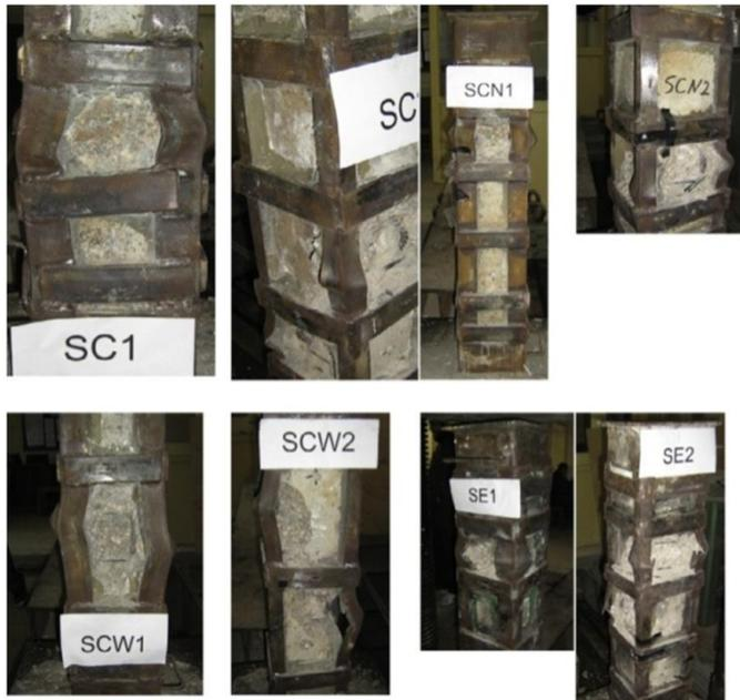
Fig 12 Fracture of weld in HS and VS
