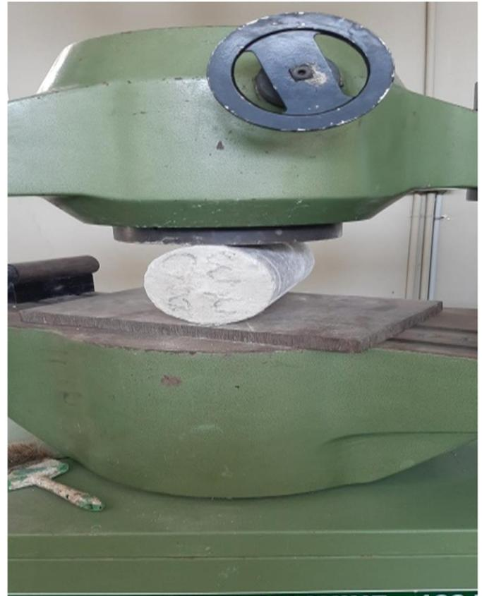
**Fig. 7 Splitting Tensile Strength Test**
