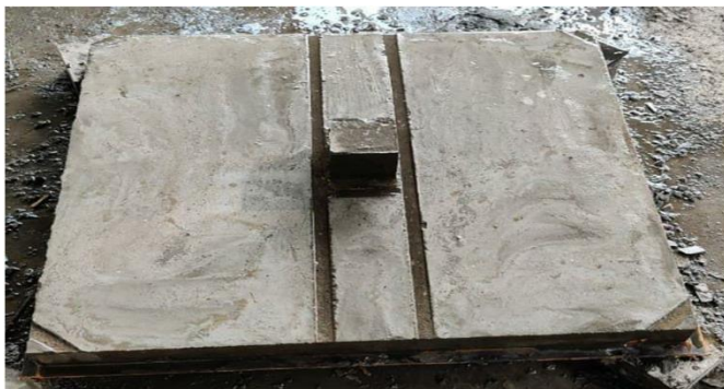
Figure 4: RC Slab Specimen
