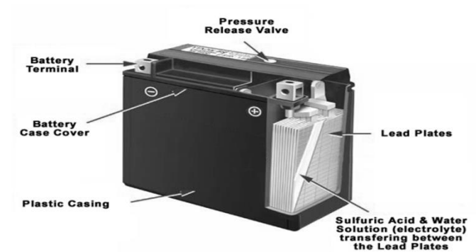
Fig: 4.5 Schematic diagram of Lead acid battery
