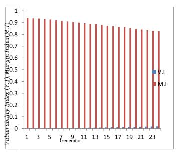
Figure 6: Variation of Vulnerability index and Margin Index versus Generator.
