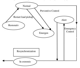
Figure i: State Transition Diagram of a Power system
