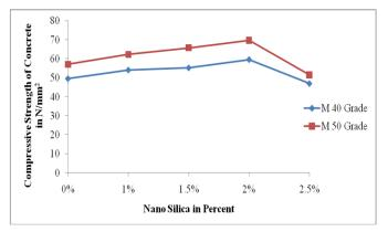
Figure 1.Compressive strength of concrete by using nano silica
