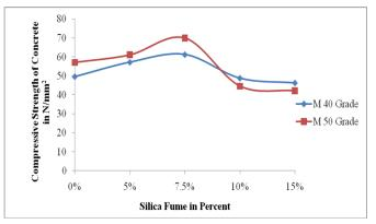
Figure 2. Compressive strength of concrete by using silica fume
