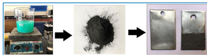
Figure 1. Synthesis and coating process of Zn/Ni nanocomposites
