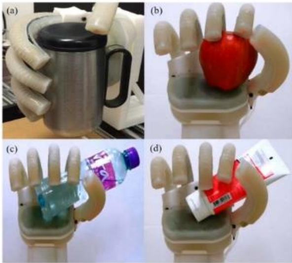
Fig 6: Grasp demonstrations: (a) a hot water cup. (b) an apple. (c) a cylindrical water bottle and (d) a lotion tube.
