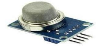
MQ-6 gas sensor is capable of detecting LPG and Butane. It's operating voltage is
