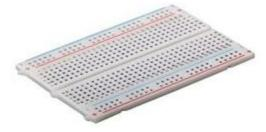
It is a construction base for prototyping of electronics. Most of the breadboard we use today are made of white plastic and it is pluggable. It was designed by Ronald J. Portugal in 1971.
