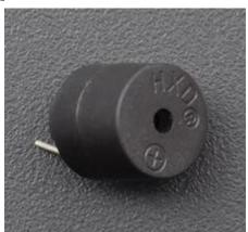
Buzzer is an audio signalling device which makes buzzing sound. It can be used as alerting device when there is some destruction happening. It act as a output device.
